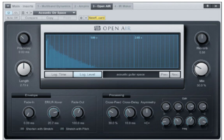
The OpenAIR plug is based on Impulse Responses from great-sounding rooms to classic hardware
