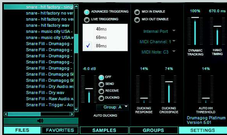
In the Settings page, latency for Advanced mode can be set to 40, 60 or 80ms
