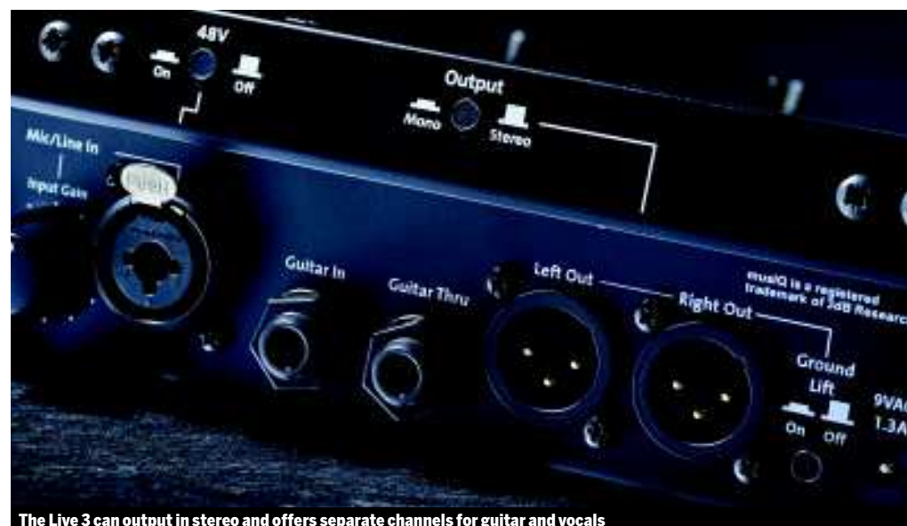
The Live 3 can output in stereo and offers separate channels for guitar and vocals
