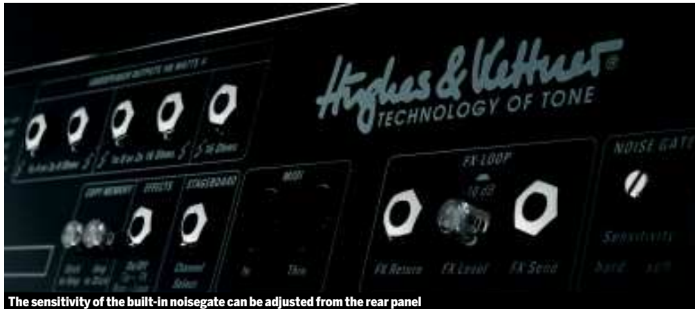
The sensitivity of the built-in noisegate can be adjusted from the rear panel
