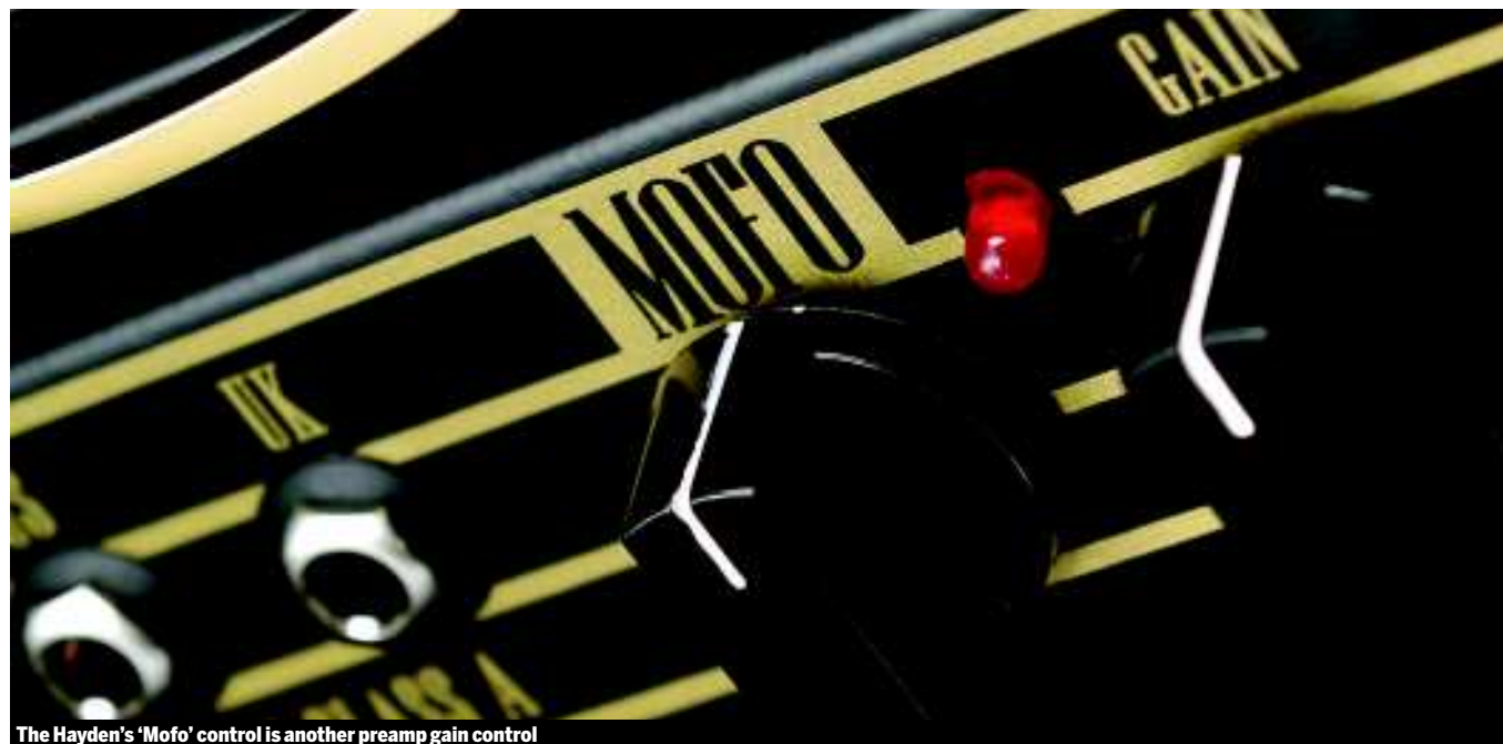
The Hayden's 'Mofo' control is another preamp gain control
