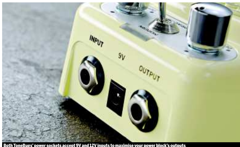
Both ToneBugs' power sockets accept 9V and 12V inputs to maximise your power block's outputs
