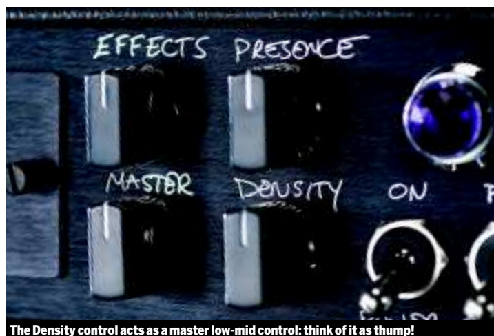
The Density control acts as a master low-mid control: think of it as thump!
