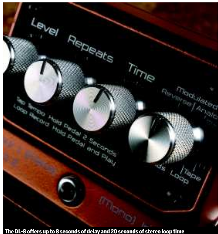
The DL-8 offers up to 8 seconds of delay and 20 seconds of stereo loop time
