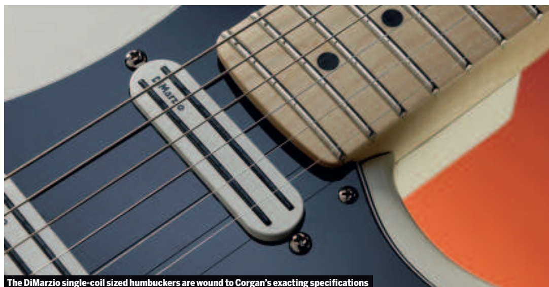
The DiMarzio single-coil sized humbuckers are wound to Corgan's exacting specifications
