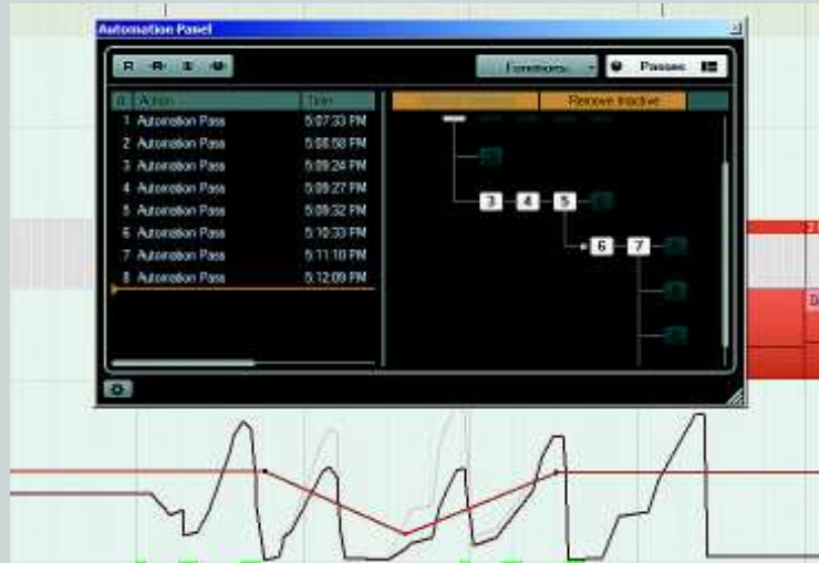
The Passes panel and Trim mode - the 'primary' automation curve appears faintly in the background
