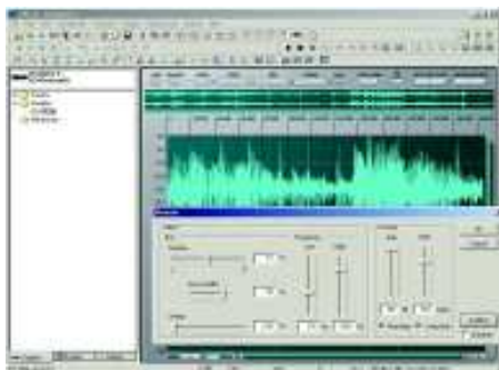
Xtractor enables you to isolate individual instruments, such as vocals, based on frequency and stereo position
