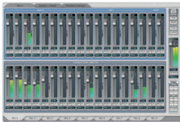
▲ You can create up to nine mixes from the 18 hardware inputs and 18 software channels
