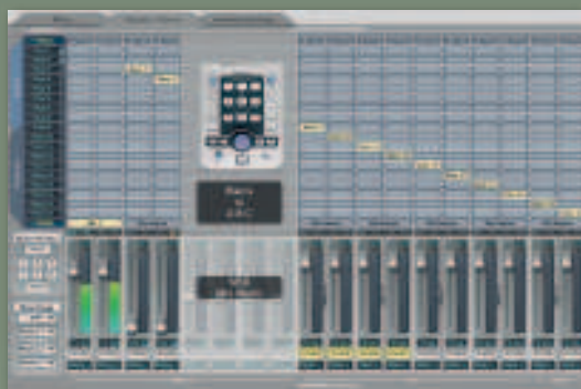
▲ Here, Mix mode is enabled on the MSR, reflected by the matrix view certainly a pain if you're trying to record more than 18 tracks with full foldback.
