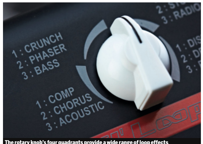
The rotary knob's four quadrants provide a wide range of loop effects
