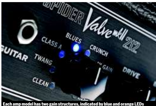
Each amp model has two gain structures, indicated by blue and orange LEDs
