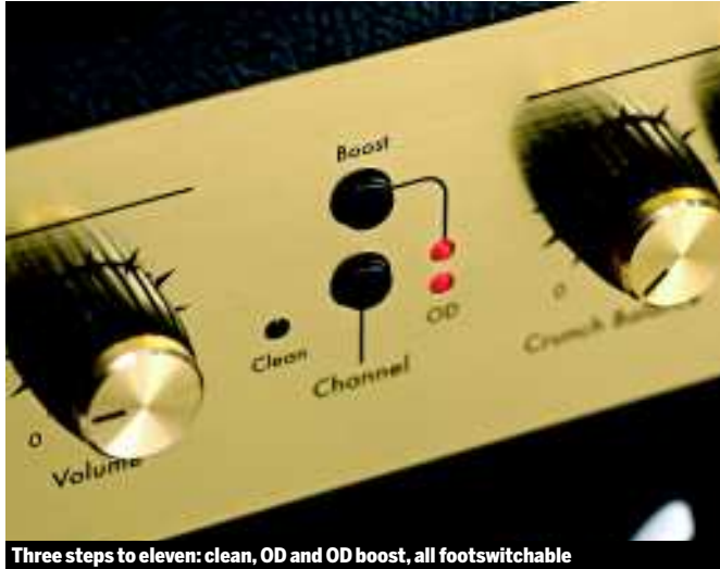
Three steps to eleven: clean, OD and OD boost, all footswitchable
