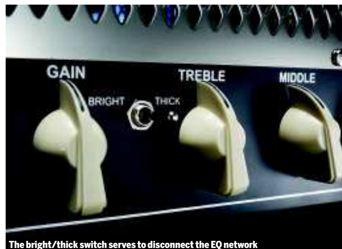
The bright/thick switch serves to disconnect the EQ network
