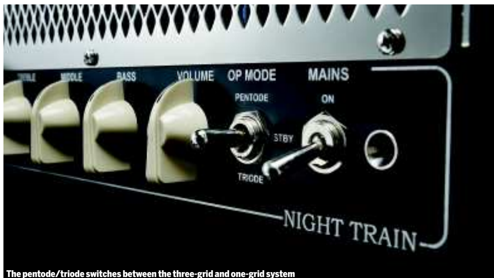
The pentode/triode switches between the three-grid and one-grid system
