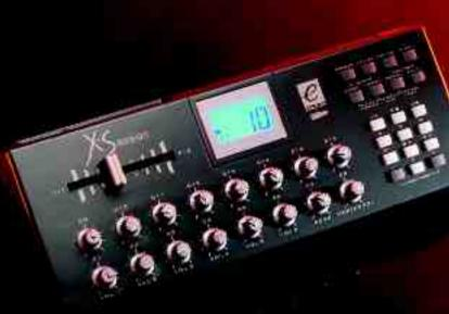
THE X-SESSION IS aimed squarely at digital DJs, but it can also serve as a perfectly good control surface for other musicians. The front panel contains one horizontal slider (for crossfades and scratchin'), a funky blue illuminated LCD display, 16 rotary
